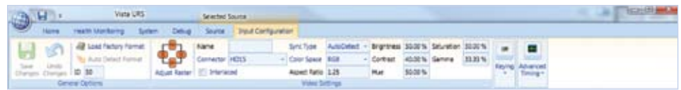
▲ The ribbon interface offers quick access to URS functionality, and contextual tabs show only relevant information based on current application selections.
